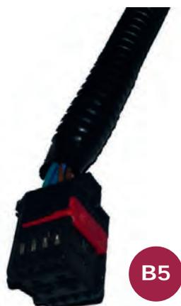
**Figure 6 - Termination of the connection harness**
