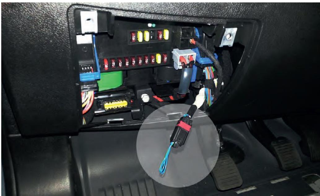
**Figure 3 - Passenger compartment fuse box**
