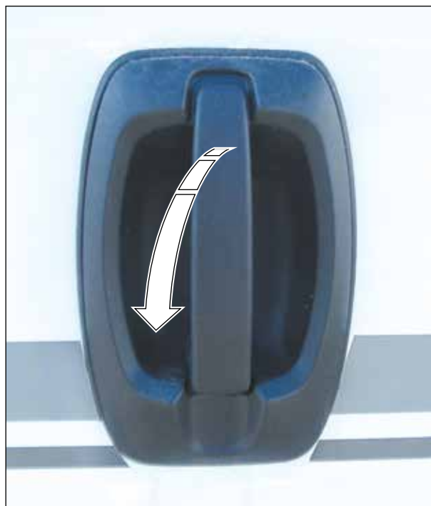
Fig. 18 Opening/closing sliding door from outside
