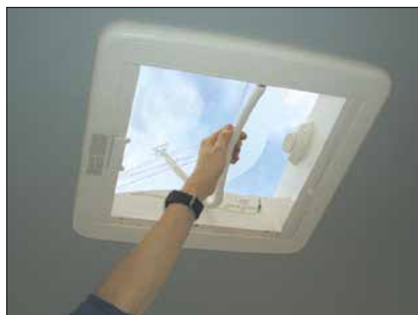
Fig. 27 Mini-Heki: Adjusting the glass dome
