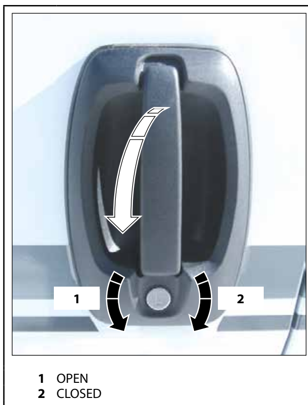
Fig. 16 Opening and closing the driver's cab door from outside
