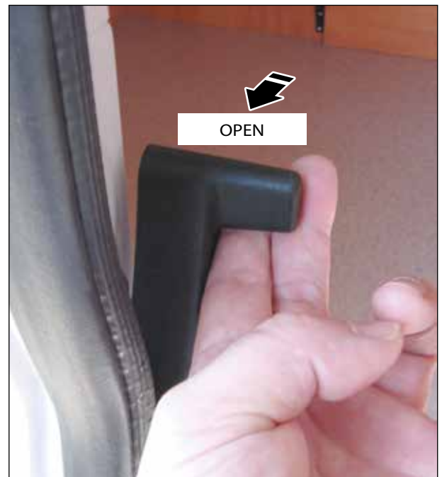
Fig. 22 Opening/closing second wing of two-wing rear door from inside
