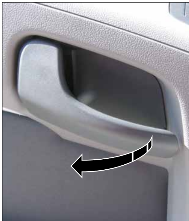
Fig. 17 Opening/Closing the Door from Inside
