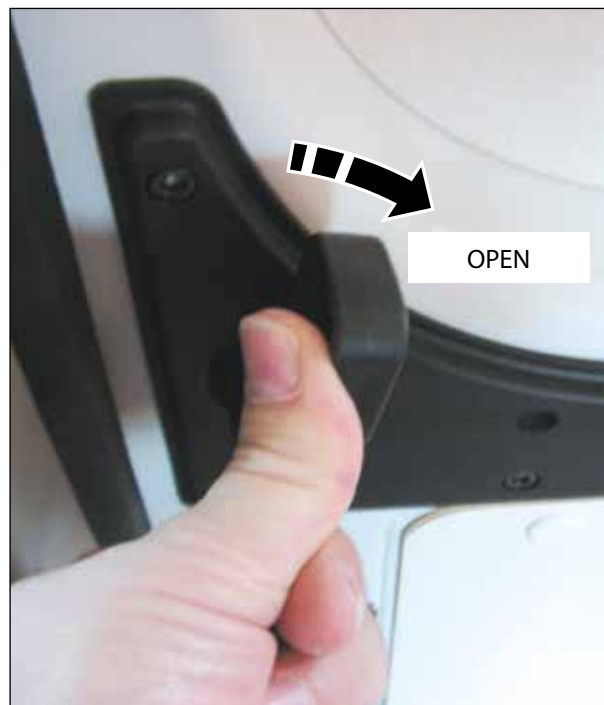
Fig. 19 Opening/closing sliding door from inside
