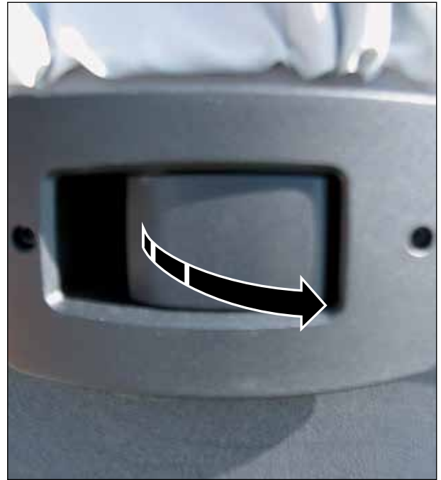
Fig. 21 Opening/closing first wing of two-wing rear door from inside
