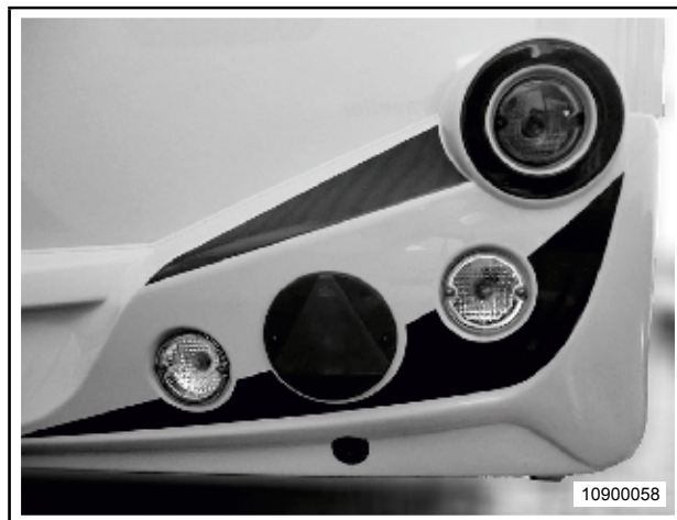
Fig. 88 Replacing lamps on the rear light holder
