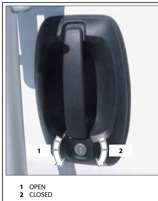
Fig. 20 Opening/closing first wing of two-wing rear door from outside
